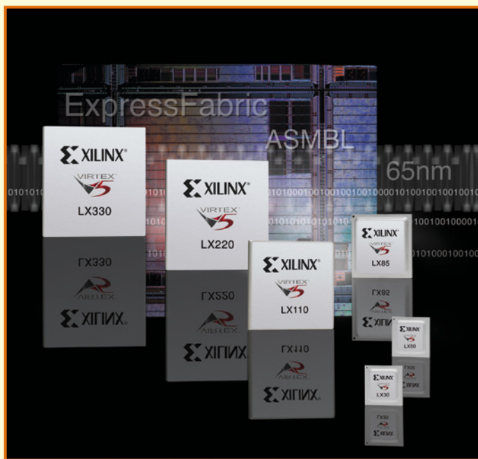
Fig. 7 - Xilinx Virtex-5: le prime FPGA in tecnologia triplo-ossido a 65 nm con processore PowerPC440, end-point PCIe ed Ethernet MAC embedded.
