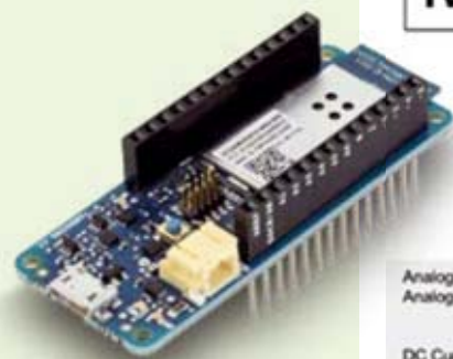
Fig. 1 - Scheda MKR1000 e relativa pin-out.
