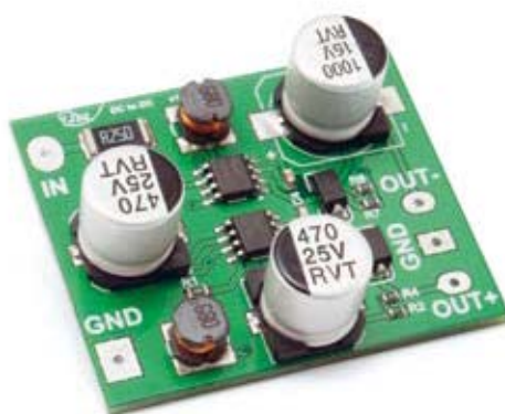
→ Fig. 13 Il converter 2846-CONVDCDC5V12V.
