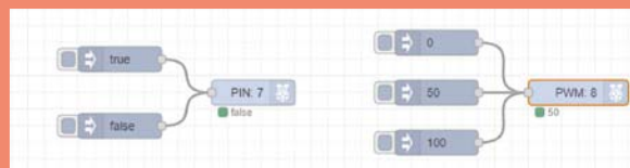
Fig. 5 - Test digital output e PWM.
