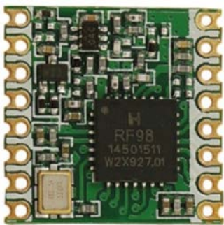
Fig. 1 - La breakout board HopeRF RFM95W.
