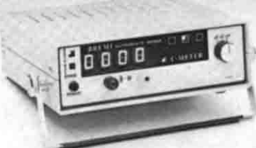
Capacimetro Digitale Mod. BRI 8004: 1 pF - 9999 \mu F
