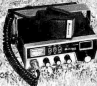
rtx mobile 5W AM 40 canali mod. 150 M
