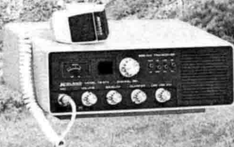
rtx base 5W AM, 15 W SSB 120 canali (40ch. AM - 40ch. LSB - 40ch. USB) mod. 76-874
