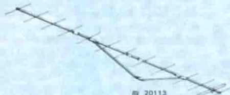
20113 12 ele. 144-146 MHz 16.5 dB 2 x 18° 2 x 23° 20 dB 50 ≤ 1.2 4.85 m
