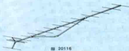
20116 18 ele. 144-146 MHz 16.5 dB 2 x 18° 2 x 17° 22 dB 50 ≤ 1.2 5.4 m
