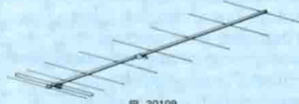
20109 20109 Portable 9 ele. 144-146 MHz 13 dB 2 x 18° 2 x 23° 15 dB 50 ≤ 1.2 3.2 m
