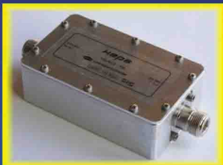
Low Noise Downconverter 2.4 GHz - 144 MHz
