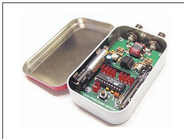
Fig. 3 - Wattmetro- SWR meter by KD1JV, montaggio "tipo Al-toids"
