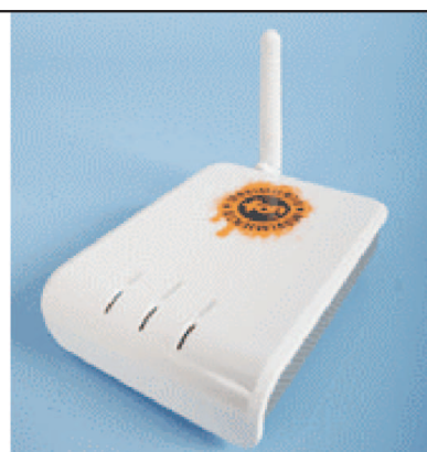
Fig.4b - Router/AP La Fonera
