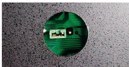
Foto 5b - Jumper backup.
