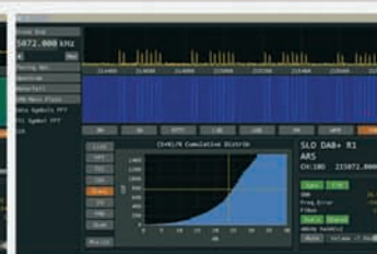
DAB+ decoder / TII spectrum and SNR stats
