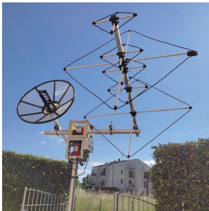
Foto 8 - Cubical Quad Dual Band VHF-UHF e monobanda 6 elementi UHF by IZ5RZR
