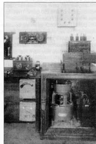
A typical early 1/2kW wireless station designed for cargo ships with motor alternator under the desk and spark transmitter above. Courtesy: Bodleian Library, University of Oxford
